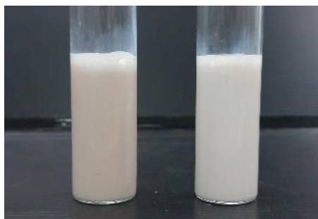
Fig. 3 Colloidal stability of TE1 formulation (left) and TE2 formulation (right)
